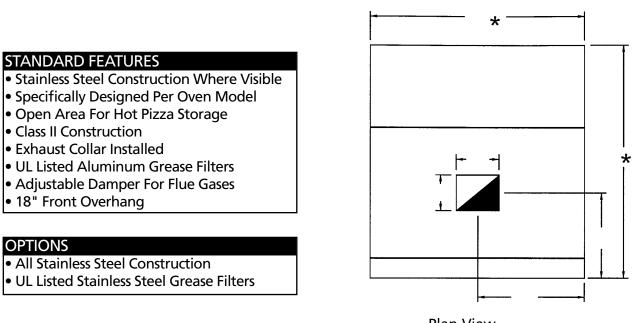
Plan View (See reverse side for larger drawing) \* OVEN MODEL NUMBER OR SIZE REQUIRED BEFORE MANUFACTURE
